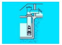
If the water level on the outlet side of the pump varies considerably flap valves can be installed.
