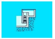
Suitable where the liquid is pumped to a tunnel, channel or basin with a water level that is nearly constant so that shutoff devices are not required.
