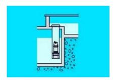
If the pump is to work in combination with a siphon or a discharge line, a pressure-tight discharge elbow must be used.
