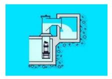
If odors require a closed system, this arrangement can be used with a free discharge, as shown, in order to prevent from water backflash.
